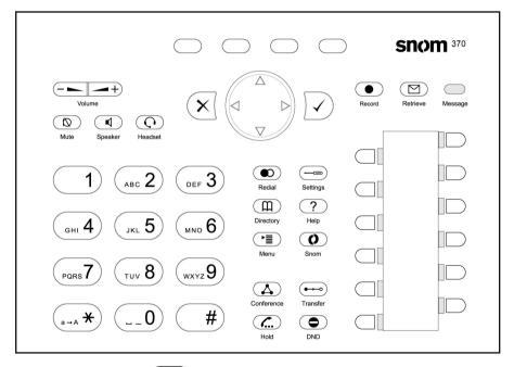
Use the MENU key E to call up the main menu. To cancel actions or input, use the CANCEL key K. The ENTER key  $\fbox{K}$  confirms actions, selections and inputs. For navigation, use the large round navigation key in the middle.
